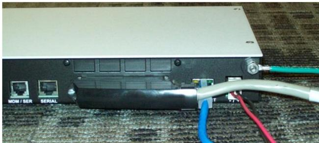
Figure 5 – Typical WS1800 with 50-pin cable connection, standard power unit shown
