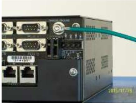
Figure 2 – Connecting Earth Ground
