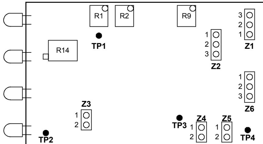
**Figure 3-8 VFCT 4- Through 8-kHz Modem Board**
