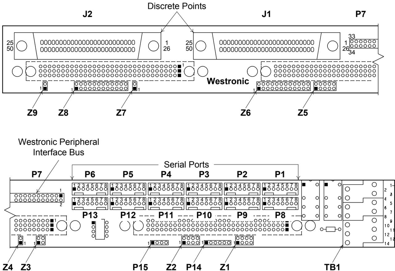
Figure 3-9 WS2000 Backplane Showing Rear Connectors and Jumper Block Locations
