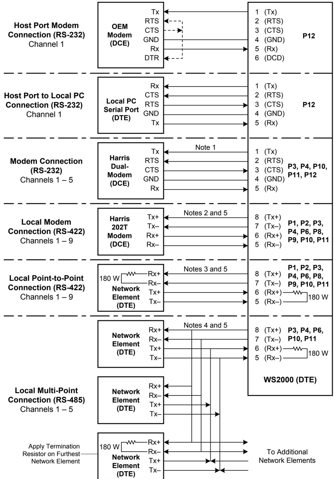
Figure 3-16 Serial Port Interface Connections for WS2000
