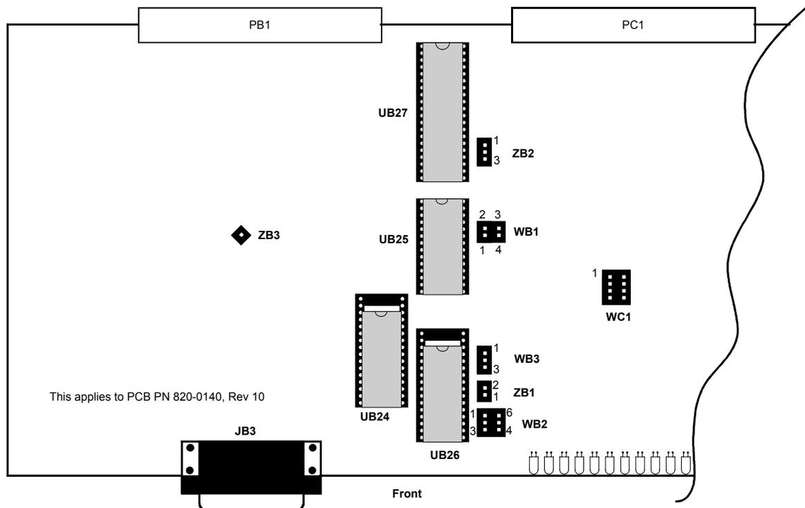
Figure 3-5 Strap Arrangements for Type 3 main Board
