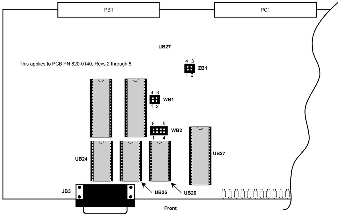
**Figure 3-3 Strap Arrangements for Type 1 main Board**
