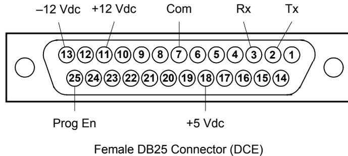
Figure 3-13 Front-Panel Connector JB3
