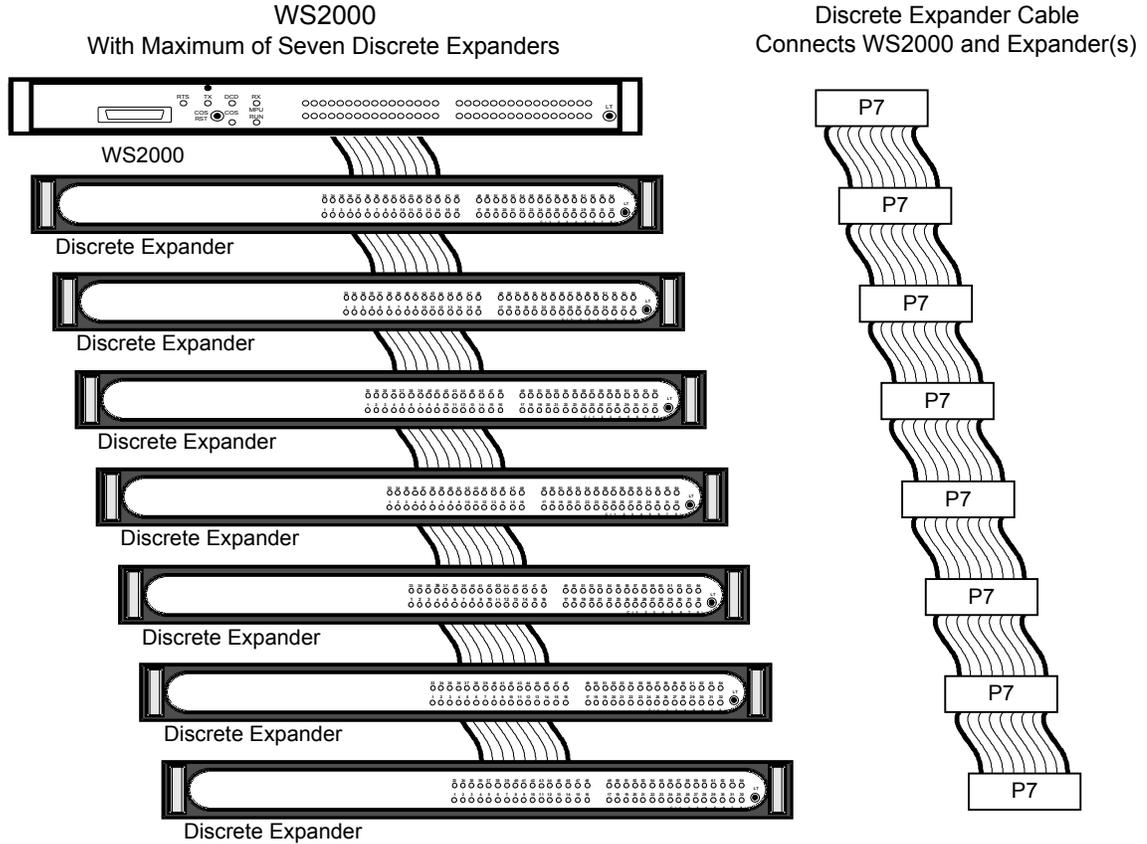
**Figure 3-18 WS2000 to Discrete Expander Interface Connections**
