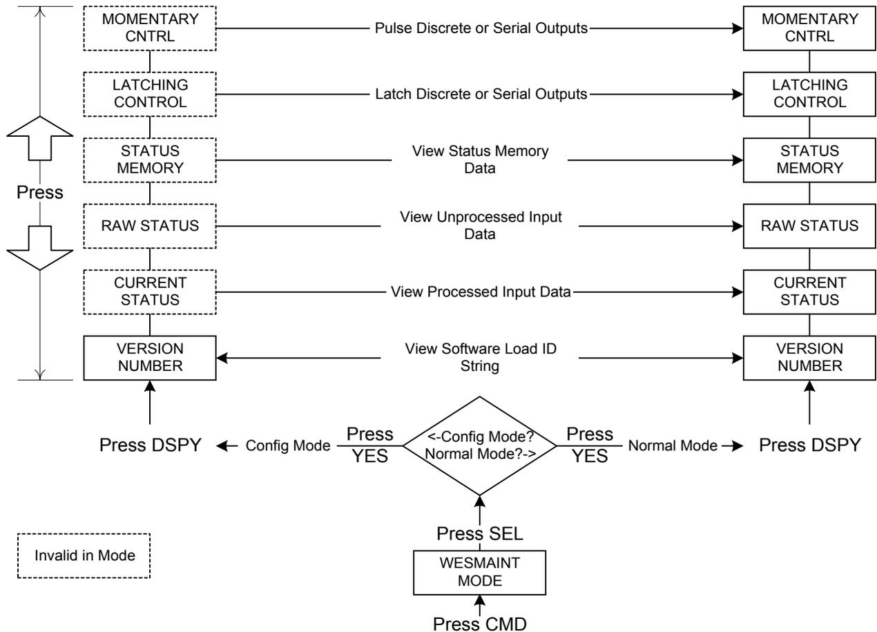
Figure 5-2 Display Function Commands
