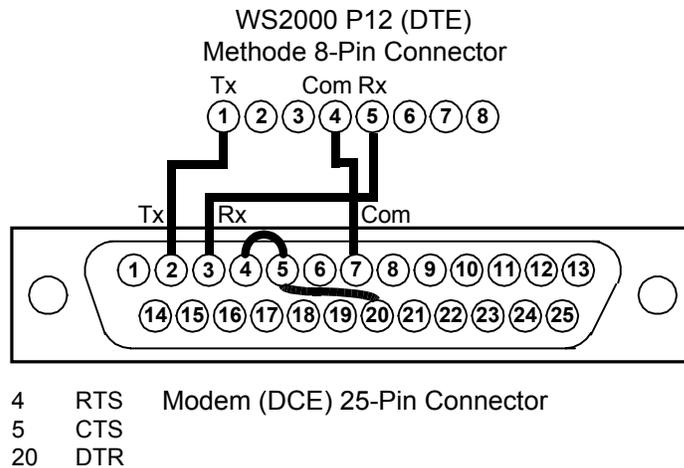
**Figure 3-15 Host Port RS-232 Modem Connections**
