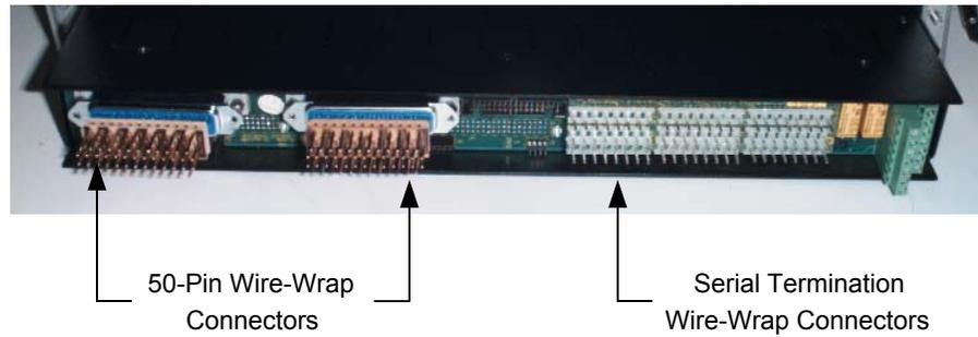
**Figure 3-31 WS2000 with Rear-Access Wire-Wrap kit**
