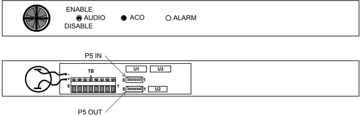
Figure 3-24 External Audible/Visual Alarm panel
