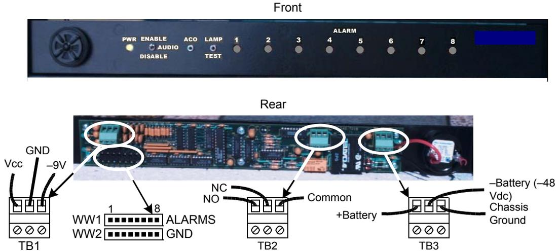
**Figure 3-25 Universal Annunciator Panel, Front and Rear Panels**
