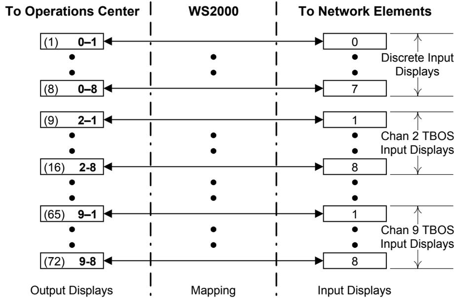
Figure 4-1 Scan (Alarm/Status) and Control Point Mapping
