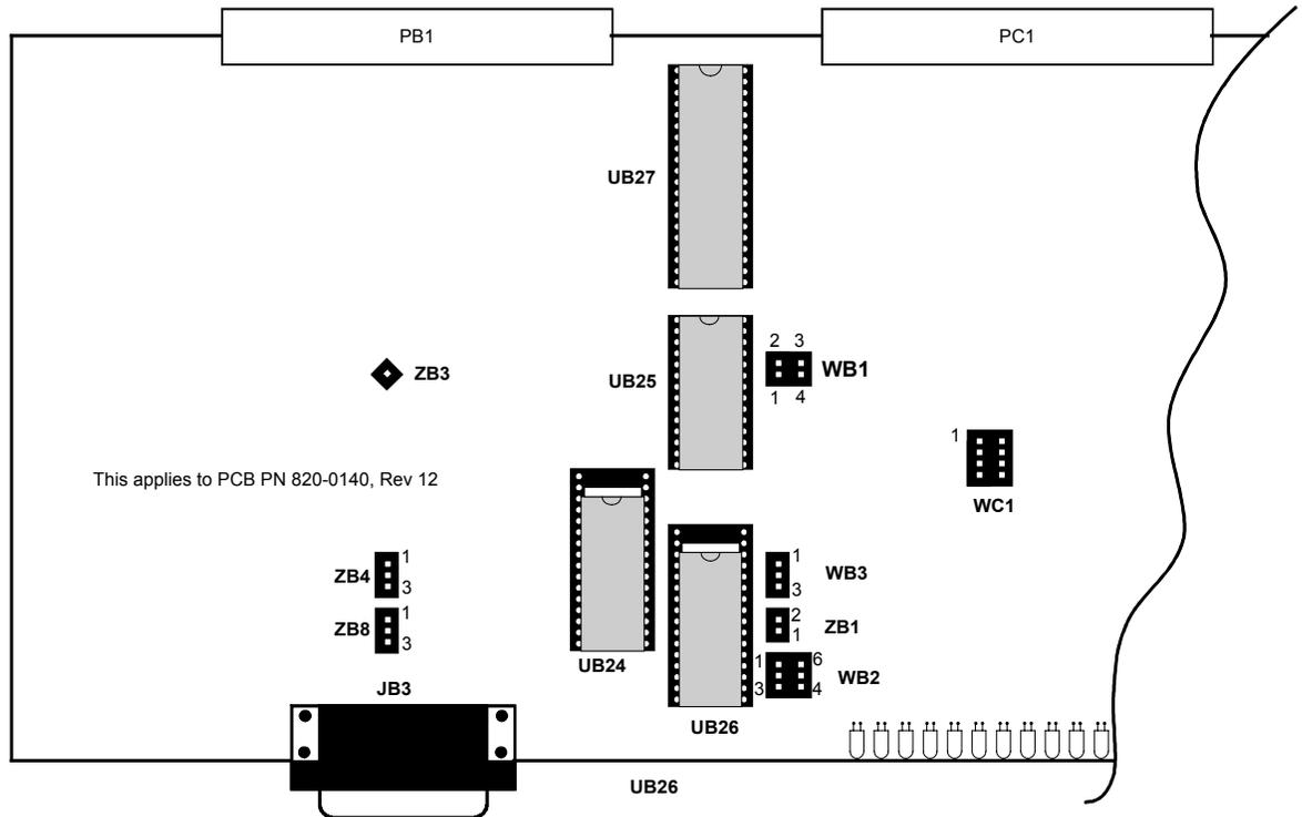
**Figure 3-6 Strap Arrangements for Type 4 main Board**
