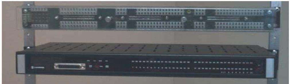
Figure 3-29 Front-Access Wire-Wrap Kit (Cover Removed)
