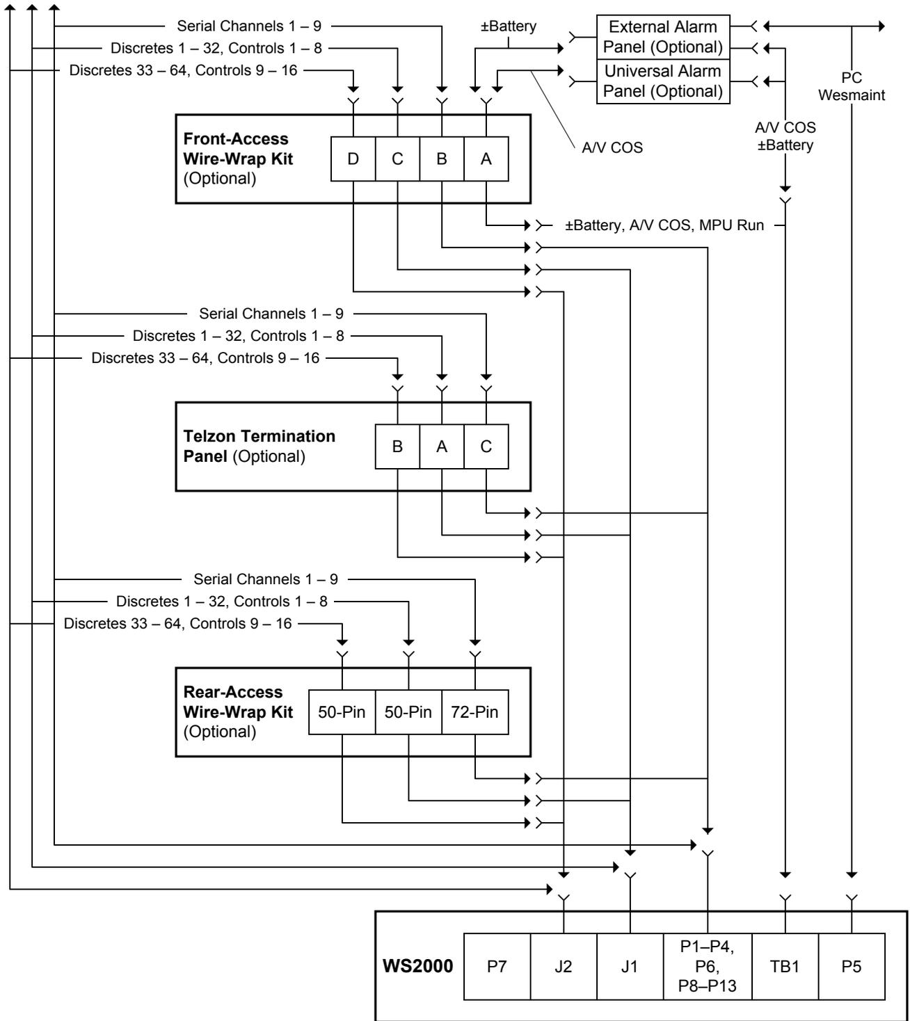
**Figure 3-12 Overview of WS2000 System Connections**
