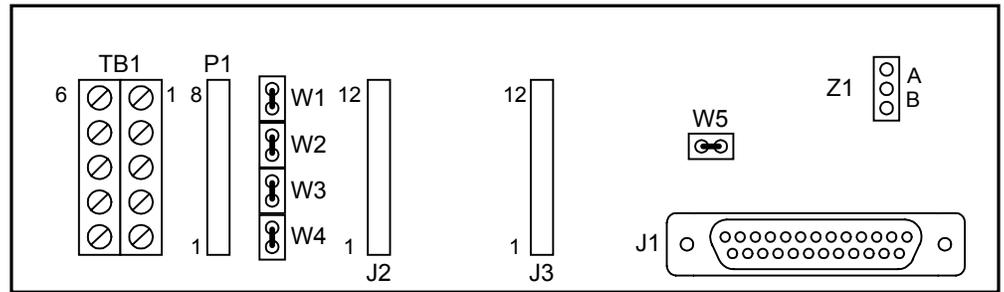
**Figure 3-21 Rack-Mount Modem Main Board**
