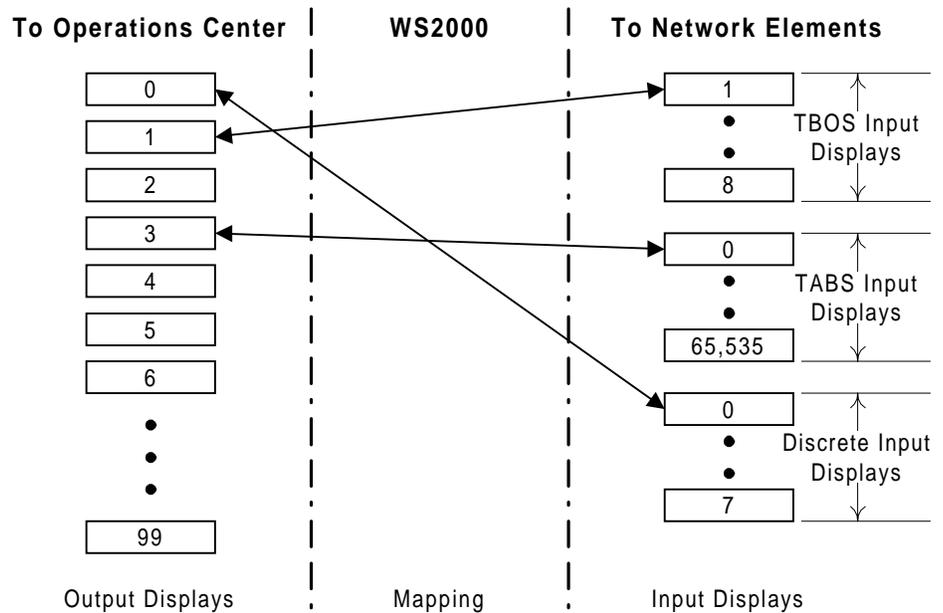
**Figure 4-5 Scan (Alarm/Status) and Control Point Mapping**
