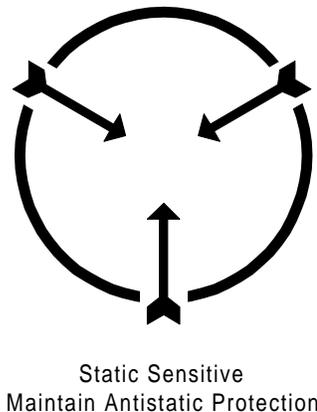
**Figure 3-1 Electrostatic Discharge (ESD) Label**
