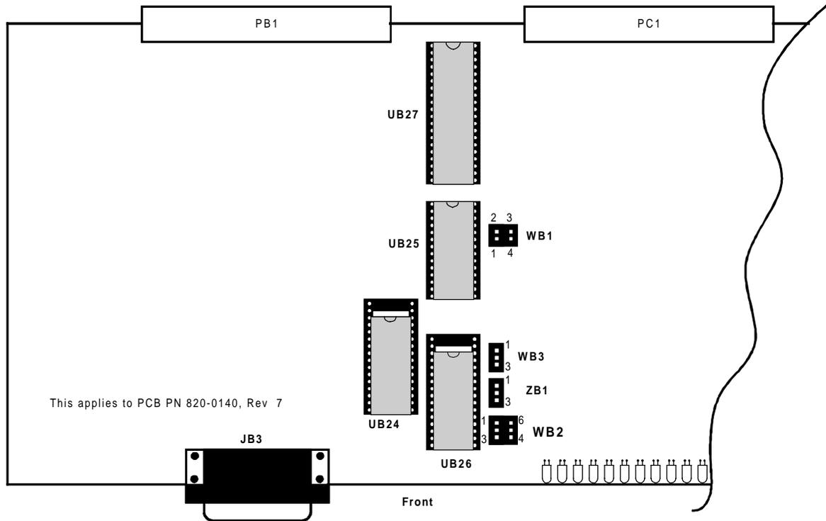
Figure 3-4 Strap Arrangements for Type 2 Main Board
