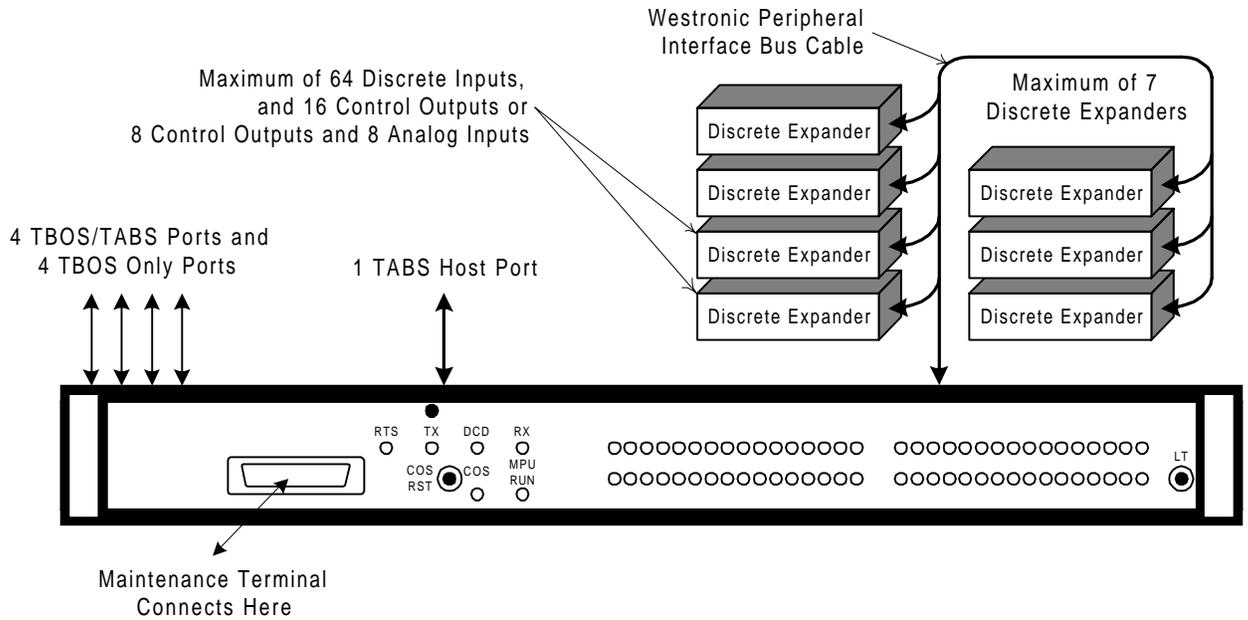
**Figure 2-3 Expansion Using Discrete Expanders**
