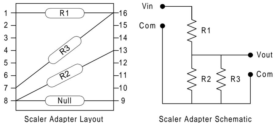
Figure 3-11 Scaler Adapter Layout and Schematic
