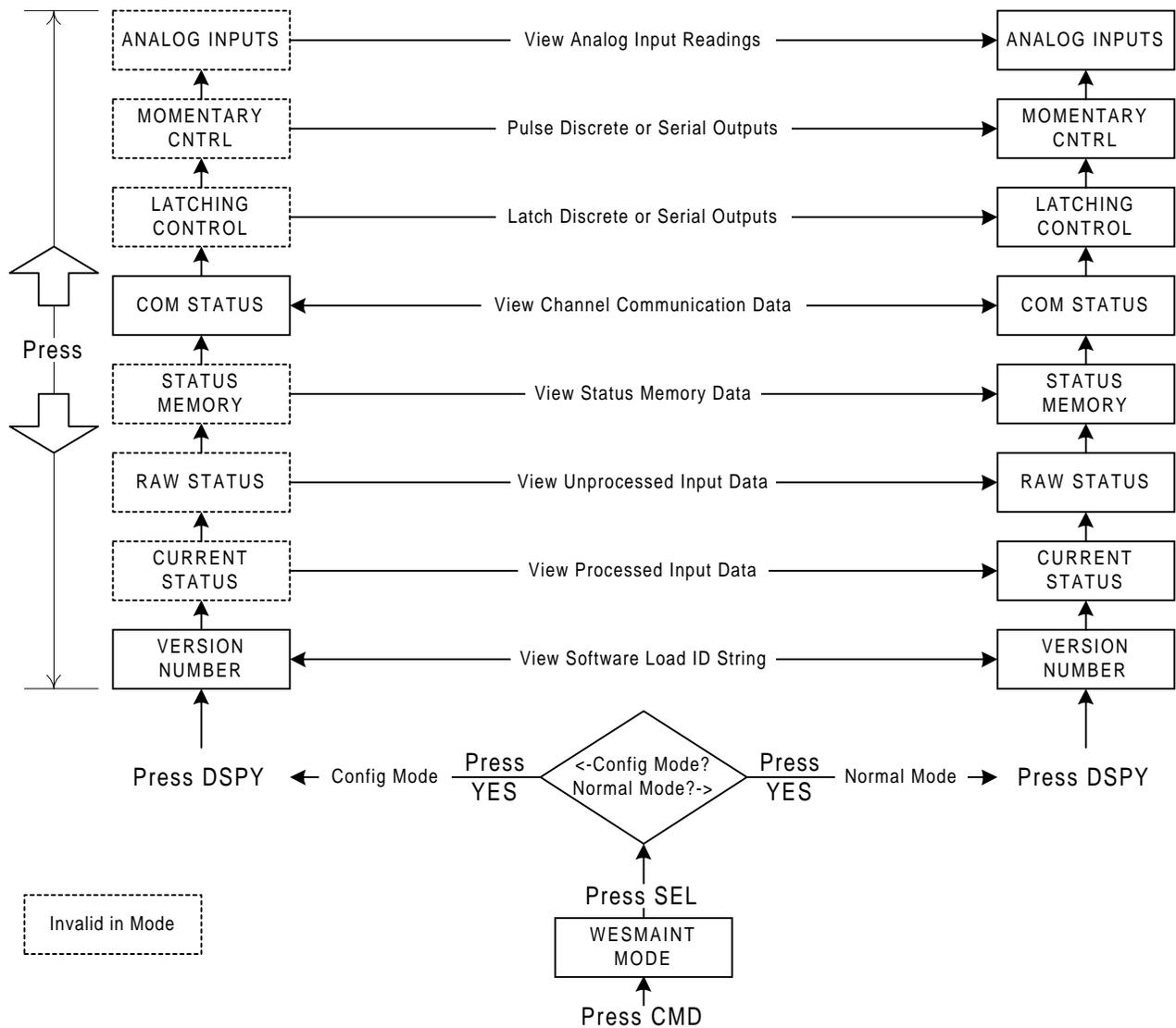
**Figure 5-2 Display Function Command**
