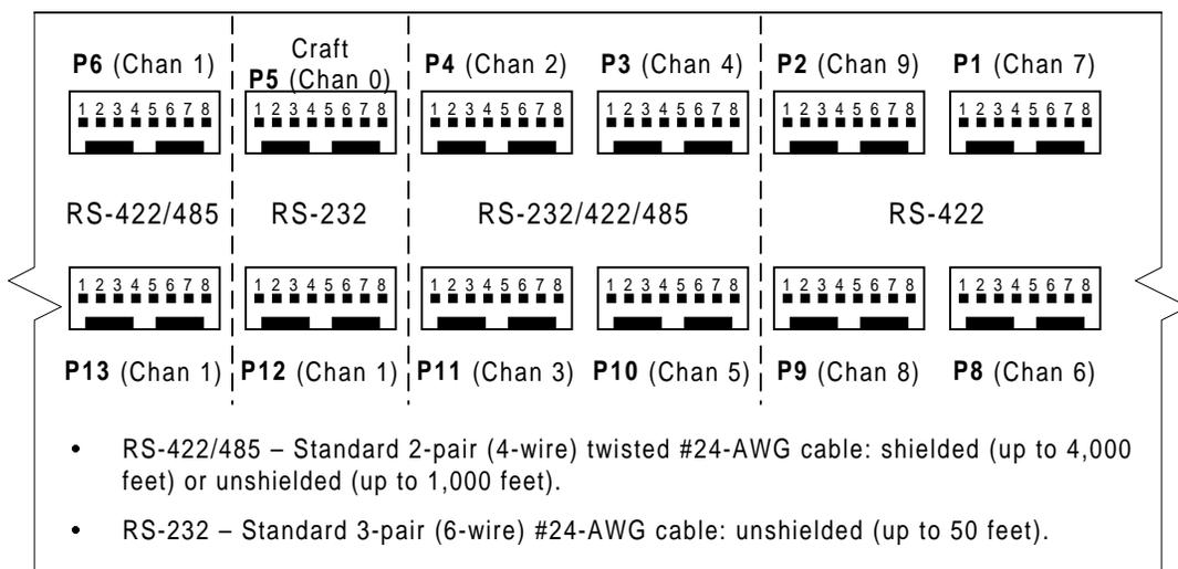
Figure 3-14 Rear View of WS2000 Serial Port Connectors (Methode)
