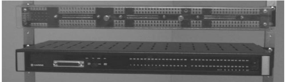
Figure 3-30 Front-Access Wire-Wrap Kit (Cover Removed)
