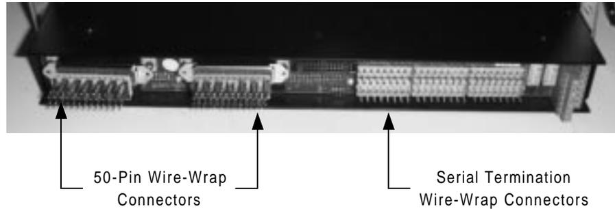
**Figure 3-32 WS2000 Dialout with Rear-Access Wire-Wrap Kit**
