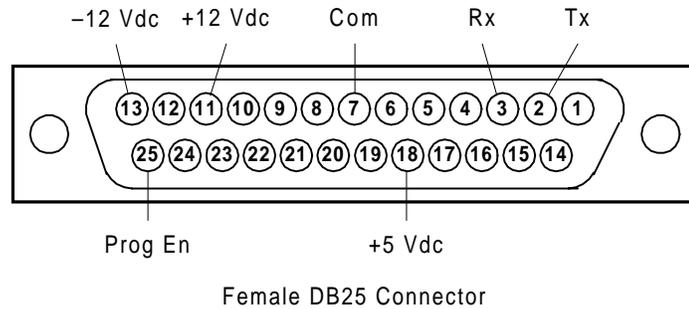
Figure 3-13 Front-Panel Connector JB3
