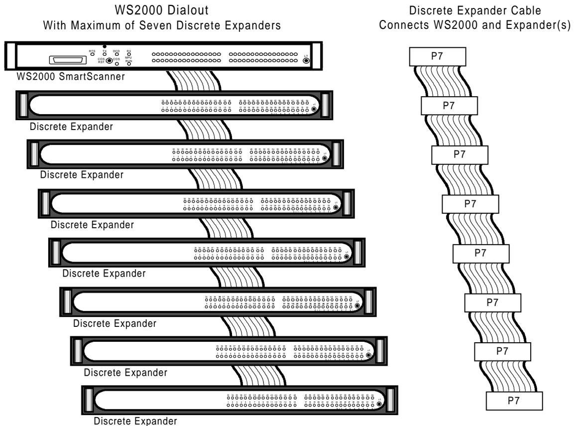
**Figure 3-18 WS2000 to Discrete Expander Interface Connection**
