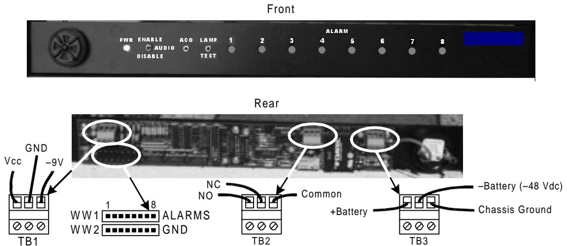
**Figure 3-25 Optional Universal Annunciator Panel Front and Rear Panels**
