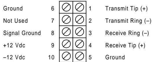
**Figure 3-22 Rack-Mount Modem TB1 Pinouts**
