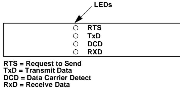
**Figure 3-20 Front View of the Rack-Mount Modem**
