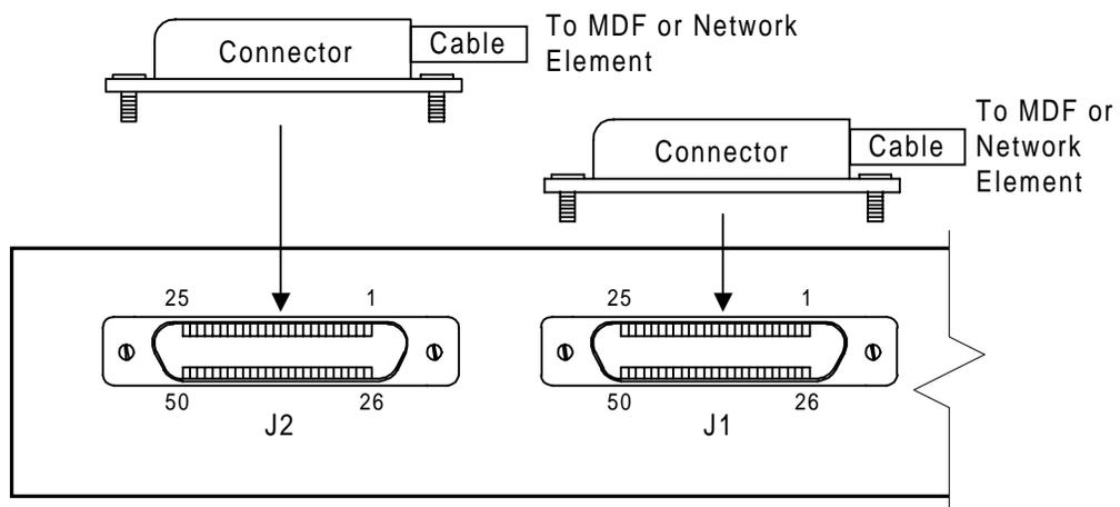
**Figure 3-17 Rear View of the WS2000 Discrete Connectors**
