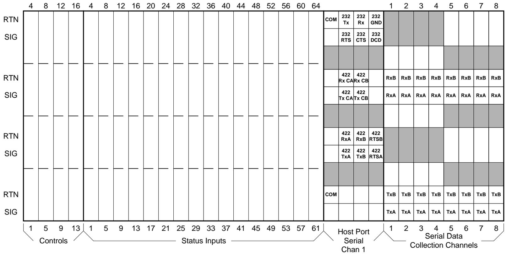
Figure 3-29 Telzon Pinouts and Functions
