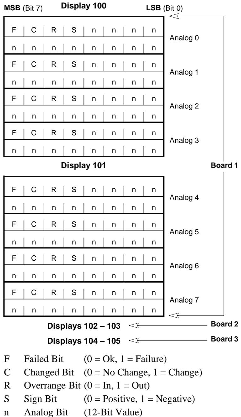
Figure 4-4 Analog Display Format
