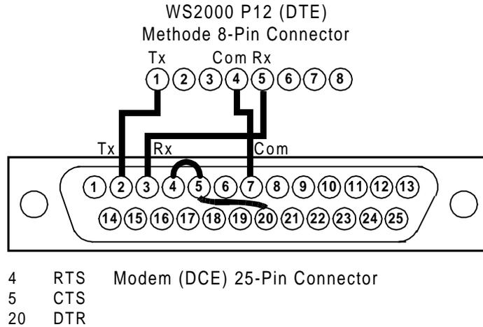
**Figure 3-15 Host Port Modem Connection for Dialout Operation**
