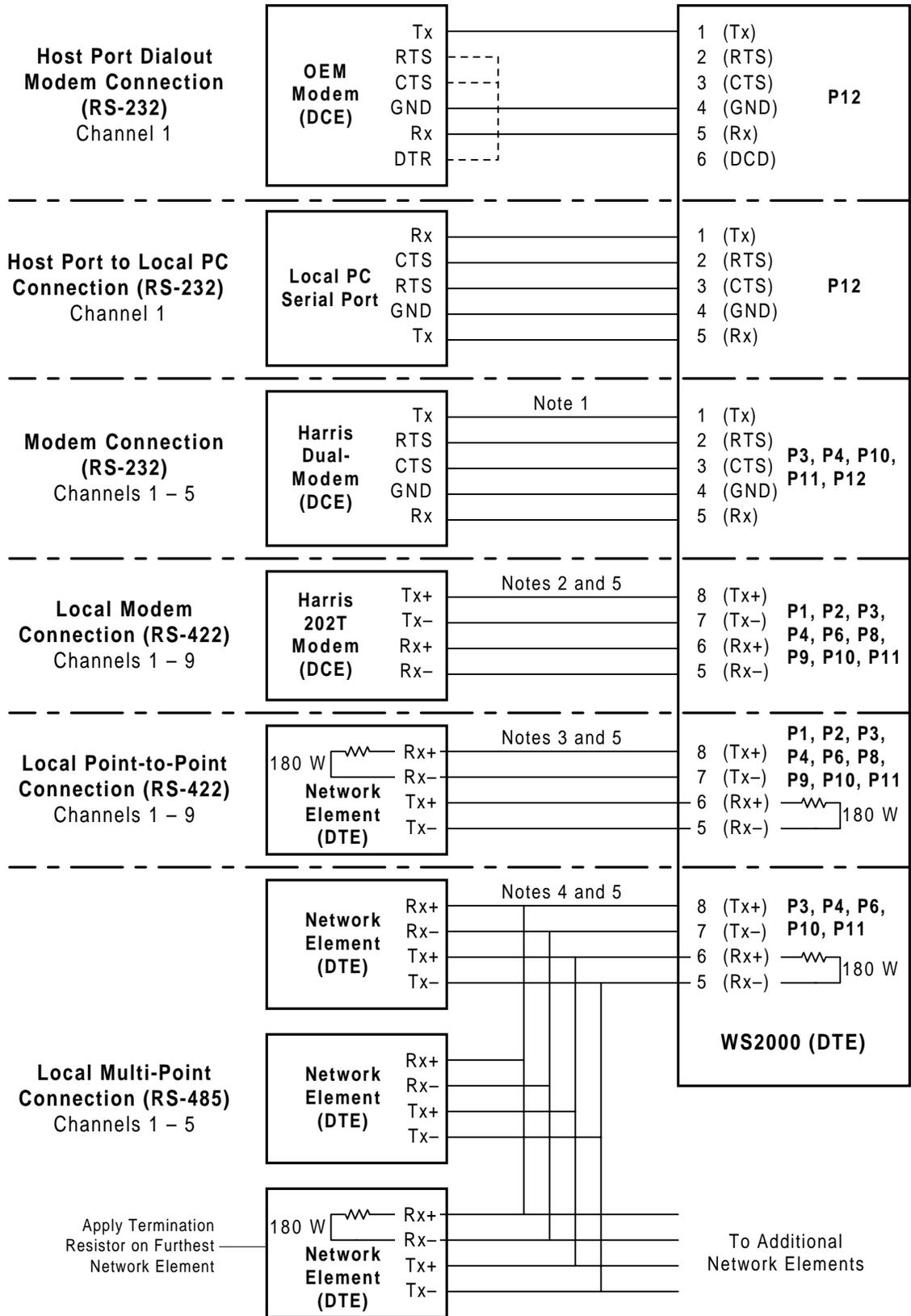
Figure 3-16 Serial Port Interface Connections for WS2000 Dialout
