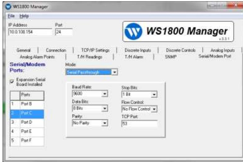
Figure 47 –Port C shown in Serial Passthrough mode
