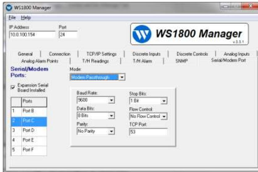
Figure 48 –Port C shown in Modem Passthrough mode
