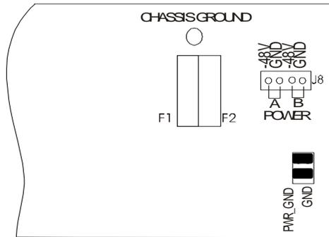
Figure 23 Power Connection and Power Fuse Location
