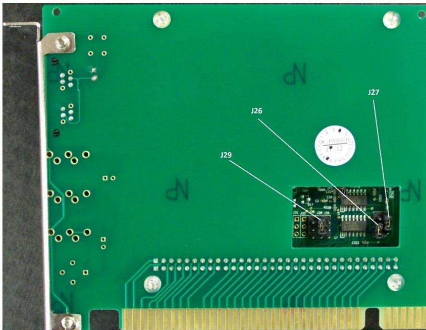
Figure 14 Modem Card Jumper Configuration
