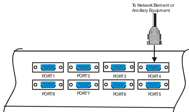
Figure 18 Serial Port Connections on the Main RTU Backplane
