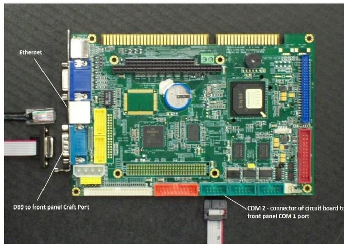
Figure 13 Connectors on the CPU Board
