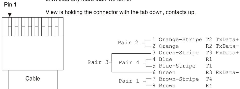
Figure 24 CAT5 Network Cable Wiring
