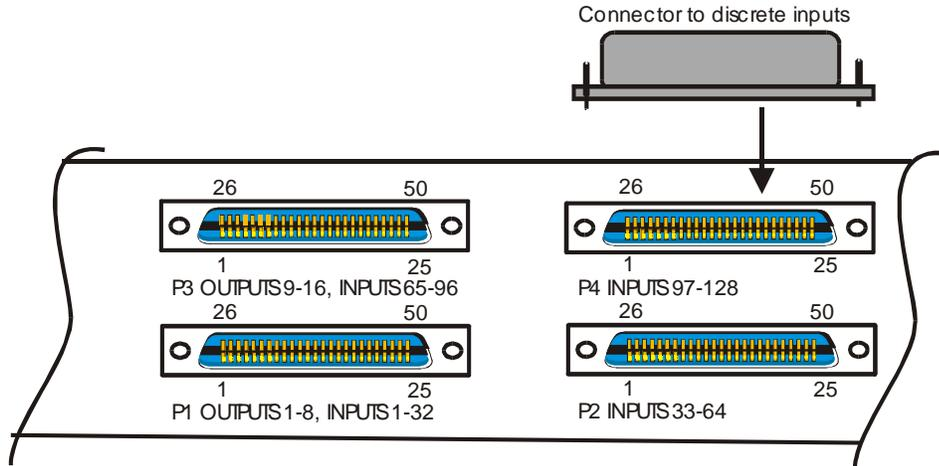
Figure 19 Discrete Input and Output Connectors
