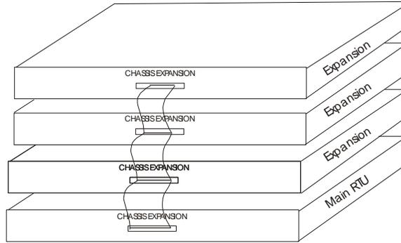
Figure 22 Expansion Chassis Configuration
