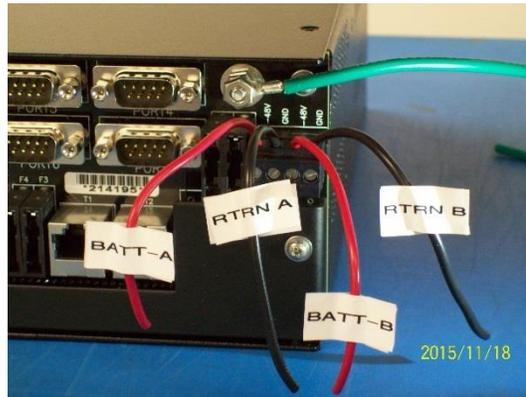
Figure 11 Backplane showing power and ground connected
