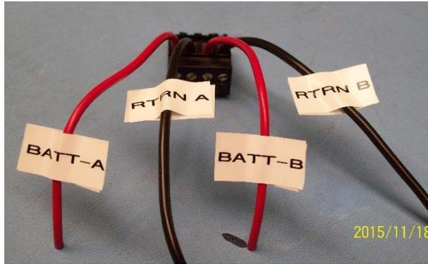
Figure 10 Wiring of DC power connector
