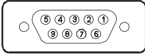
Figure 21 Front DB9 RS-232 Serial Port Connector
