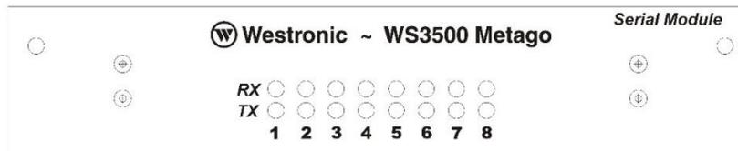
Figure 5 Serial Expansion Module Front Panel
